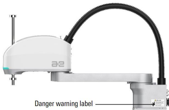
Figure 2-6 AIR6SC-750A manipulator hazard warning label location diagram
