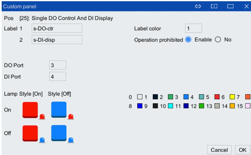
Figure 6-33 "Single DO control and DI display" Setting interface
