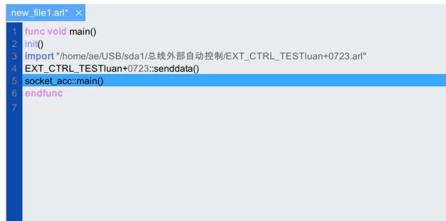
Figure 5-63 Subprogram is inserted (if it is in the same path as the main program)
