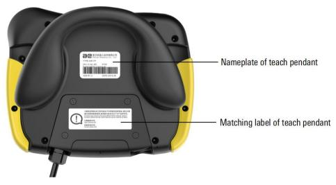
Figure 2-3 The position of the nameplate and matching label of the teach pendant
