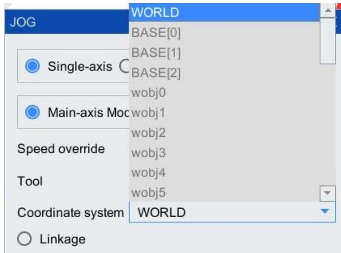
Figure 4-21 Manual reference coordinate system selection interface
