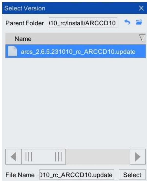
Figure 8-41 Path where ARCS upgrade file is located
