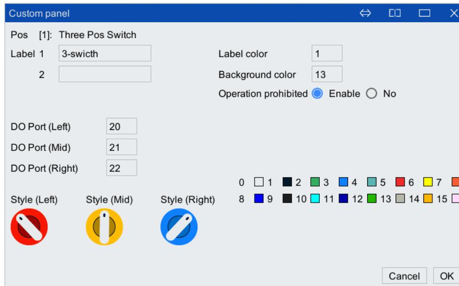
Figure 6-109 "Three pos switch" setting interface
