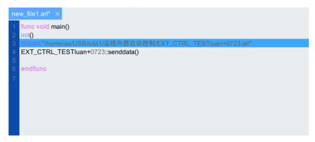
Figure 5-62 Subprogram is inserted along with its path (if it is not in the same path as the main program)
