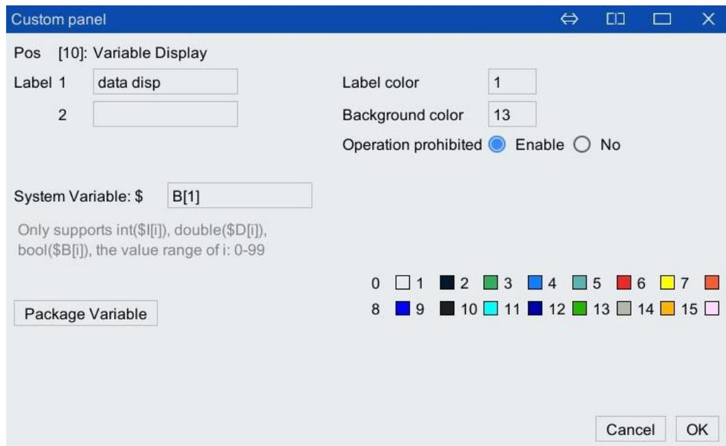
Figure 6-125 "Variable display" setting interface
