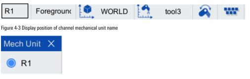
Figure 4-4 "Mechanical unit" selection interface
