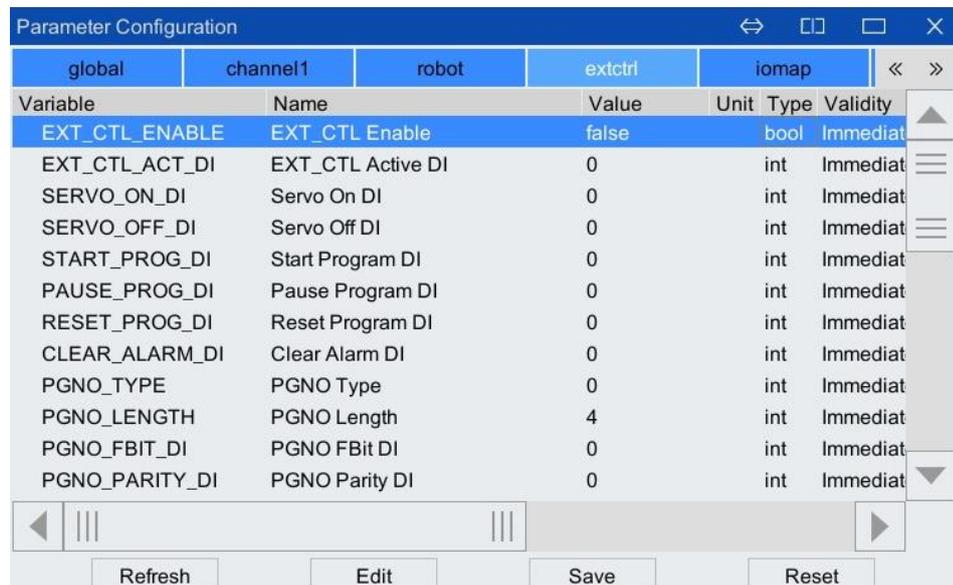
Figure 6-27 [External Control] tab in [Parameter Configuration]
