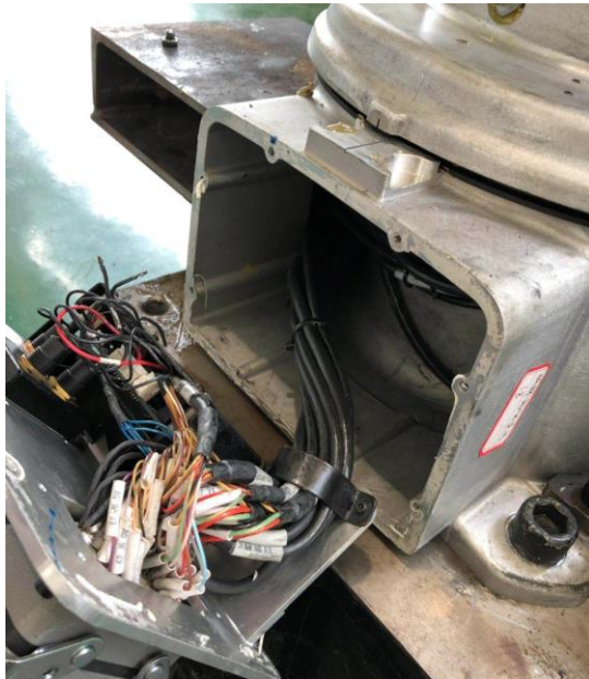
Figure 12-2 Internal cables of the base
