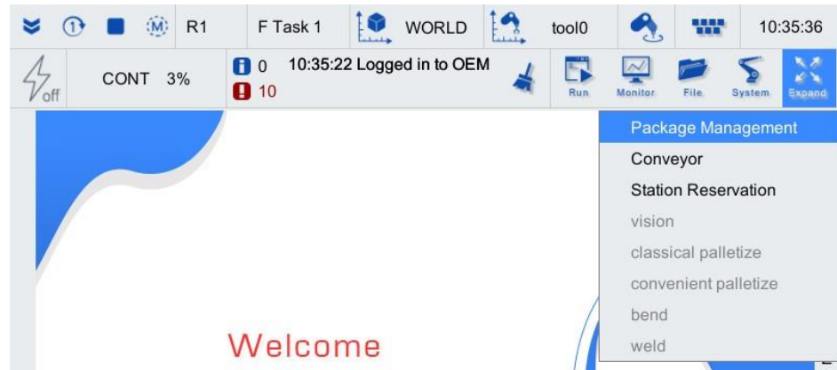
Figure 5-1 Teach pendant main interface diagram
